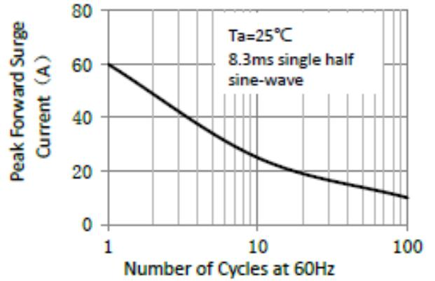
Figure 2. Maximum Non-Repetitive Peak Forward Surge Current
